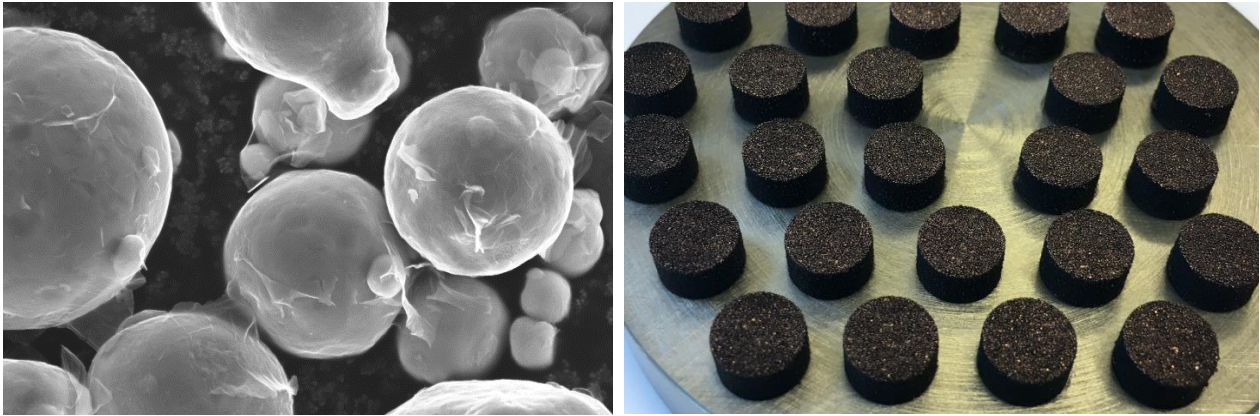
Copper powder was coated using Graphmatech's patented graphene technology. Credit: Simon Tidén / Uppsala University
